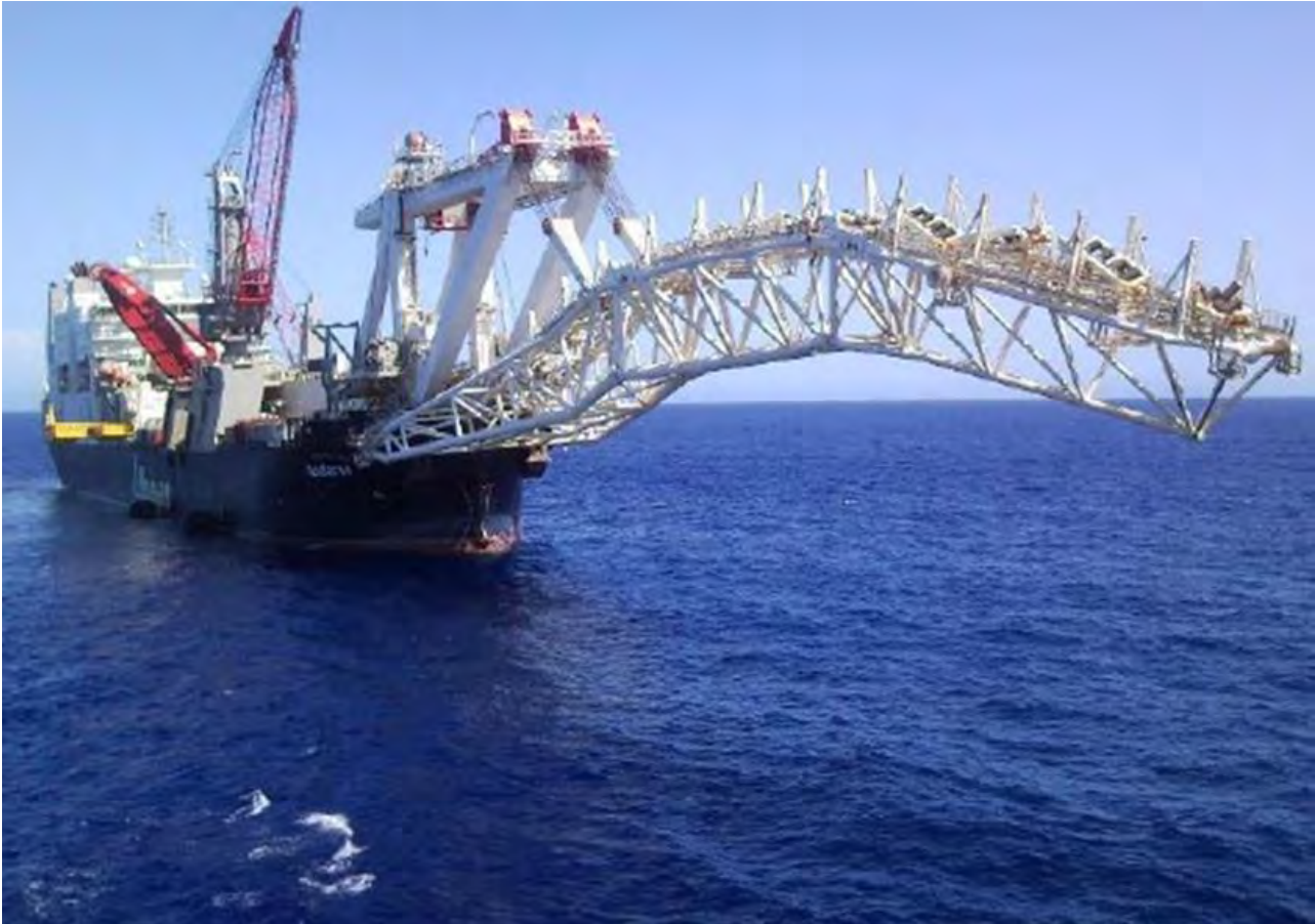
Figure 4-2: Conventional pipelay vessel
