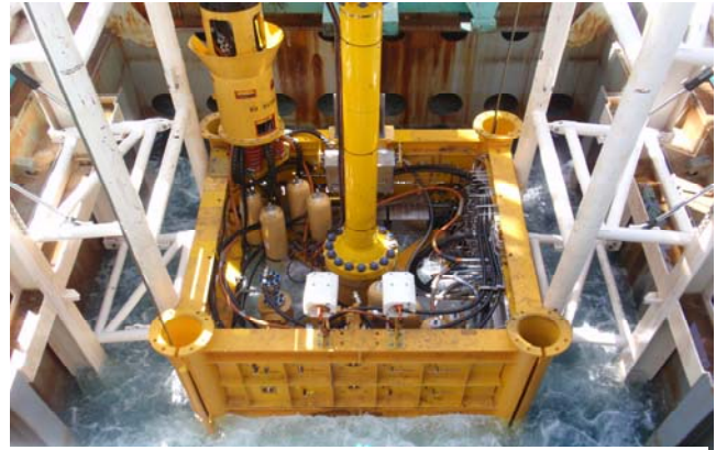
Subsea intervention device being deployed through the moonpool.
